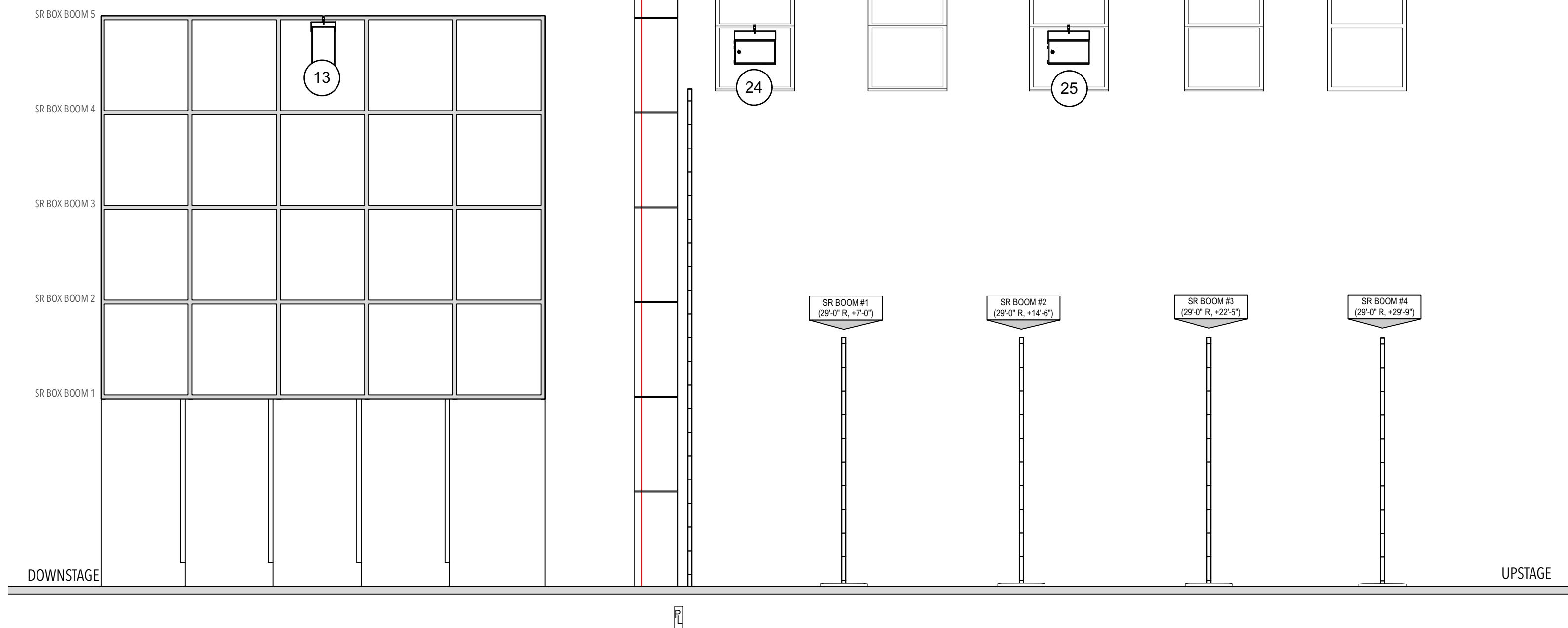
STAGE LEFT LADDERS TRIM HEIGHT TO DECK FROM BOTTOM OF LADDERS: 20'-0" US/DS POSITIONS MEASURED FROM DS SIDE OF LADDERS
